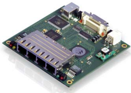
NetLink PLUS as custom specific OEM solution on GigabitEthernet base (Image: SiliconSoftware_NetLinkPLUS.tif, 300 dpi, CMYK, 13.80 x 10.80 cm)
