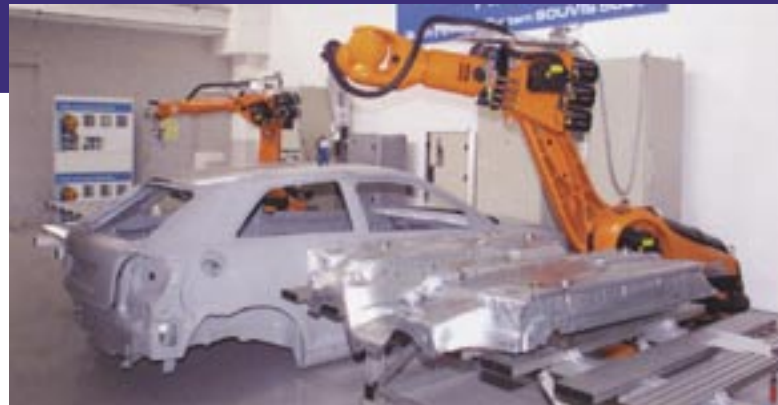
FIGURE 1. Souvis 5000 system analyzes the profile, structure, and pores of welds with a single integrated sensor.
